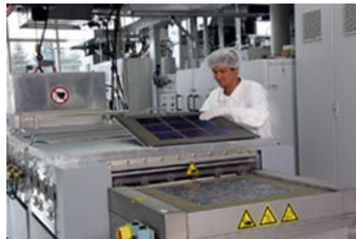
Fig.. 4: In-line installation for wet etching of silicon wafers. Fig. 5: Processing alternative: PVD-Coating. Pictures: Fraunhofer ISE
