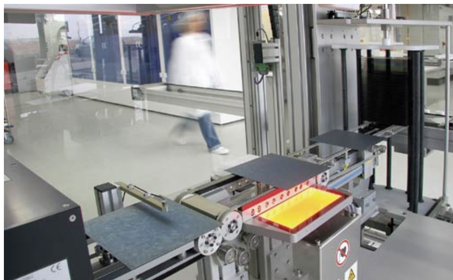
In PV-TEC every single product goes through a complete, mainly automated monitoring system – from the wafer to the finished solar cells. Photo: Fraunhofer ISE
