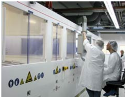
Fig.. 4: In-line installation for wet etching of silicon wafers. Fig. 5: Processing alternative: PVD-Coating. Pictures: Fraunhofer ISE
