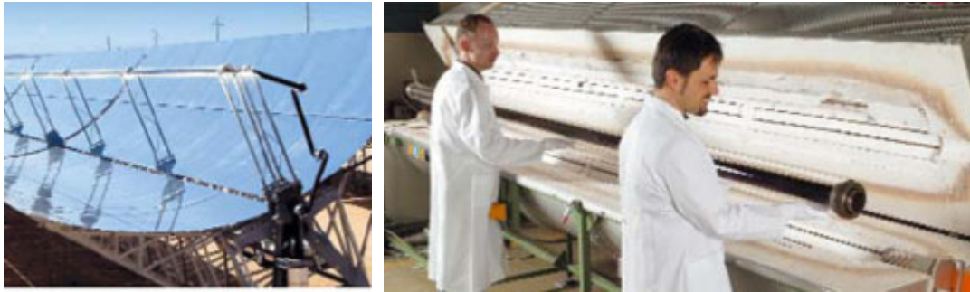
Left: A solar receiver collects concentrated solar energy. Right: SCHOTT employees in Mitterteich manufacturing and testing parabolic trough receivers. Source: SCHOTT AG
