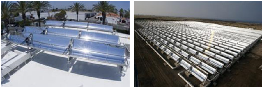
Left: microCSP system by Sopogy. Right: The world's first MicroCSP plant Holaniku at Keahole Point, Hawaii, Courtesy Sopogy
