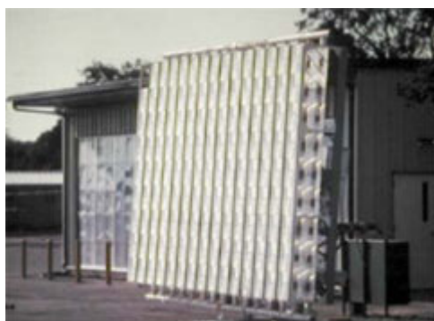
Sandia PV concentrator from the year 1976 (left), Concentrix CPV system with two-axis tracking. Sources: Sandia Labs, Concentrix Solar GmbH
