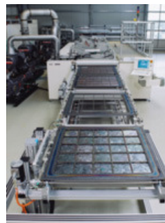
Left: Model of a turn-key solar silicon factory of the company centrotherm photovoltaics. Right: Solar cell coating system SiNA_L by Roth & Rau
