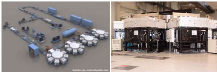
Applied SunFab production line (left) uses substrates that are four times the size of the modules currently used. A glimpse of future production of Sunfilm AG (right). Sources: AMAT; Sunfilm
