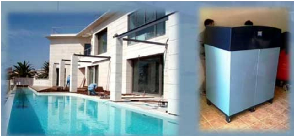
Photos: Single-family residential home in Chiclana de la Frontera, Spain. Cooling machine: ClimateWell 10. Source of power: 36 m 2 flat plate collectors. Heat rejection: swimming pool. Cooling: Distribution through chilled floors. Planning & implementation: "8'17".
