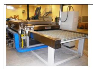
The photovoltaic panel assembling line includes 1 panel washing-machine "TRIULZI", a welding station "SOMONT", a lay-up "SOMONT", a solar simulator "PASAN", a laminator "3S", etc.
