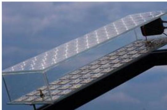
The high module efficiency was measured under Concentrator Standard Testing Conditions (CSTC), and marks the best value ever achieved for a solar photovoltaic (PV) module.
