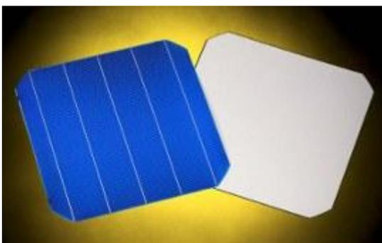
A day later, the Institute for Solar Energy Hamelin has produced a passivated emitter rear contact (PERC) PV cell with an efficiency of 21.2%, as confirmed by Fraunhofer ISE. This is the highest efficiency recorded to date for a single-junction crystalline silicon PV cell with screen-printed metal contacts. [More](#)
