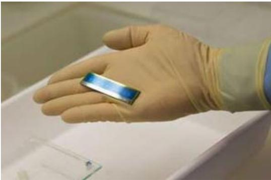
ZSW succeeded in bringing back the record to the institute with this cell's performance. Swedish researchers achieved a new best mark in June, which has now been surpassed by 0.7 percentage points. The record-setting cell has an area of 0.5 cm<sup>2</sup>, a standard size for such tests. It was manufactured in a laboratory coating plant by way of a coevaporation process that is highly reproducible in the lab.
