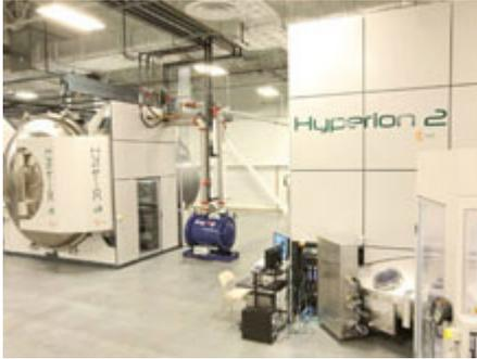
*Twin Creeks' Hyperion wafer production system allows for the production of ultra-thin, kerfless wafers*
